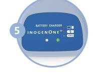
When the green light illuminates, the battery is fully charged\*.
